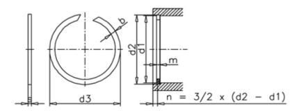
$\begin{array}{lll} b & = 5.00 \\ d1 & = 230 \\ d2 & = 233.0 \\ d3 & = 235.3 \\ Description = SB 230 \\ FN kN & = 181.00 \\ FR kN & = 52.00 \\ m min & = 3.2 \\ \end{array}$
